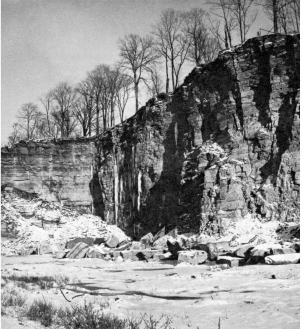
The Rockcliffe Formation in this quarry beside Highway 17 between Orleans and Cumberland shows fairly massive, sandy beds. Large blocks of sandstone are left on the quarry floor after the more shaly fraction is taken away for fill and road construction.
