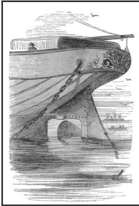
FIG. 1. SCREW STEAM-VESSEL, SHOWING THE FAN.
