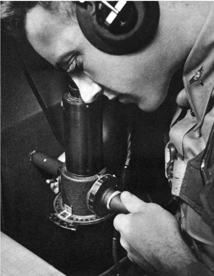
Navigation cadet looks through the driftmeter
