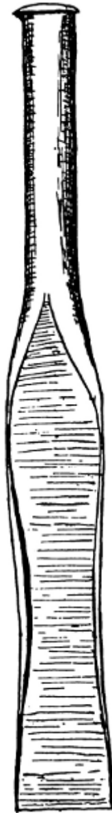
FIG. 54.—Copper chisel with “flanged” blade from the tomb of Hetep-heres, the mother of Cheops.
