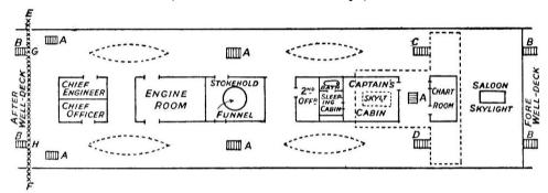
Dotted lines show rough positions of boats, and limits of bridge overhead.
