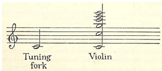
Fig. 32. The tuning-fork only sounds single pure tones. A single note of the violin, on the other hand, sounds a whole chord of pure tones—hence the richness and fullness of good violin tone.
