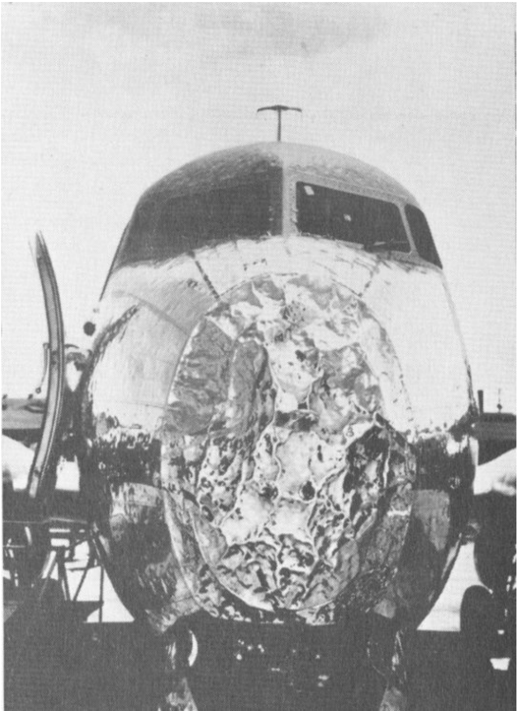
Thirty seconds of flight through a hailstorm did this to a
