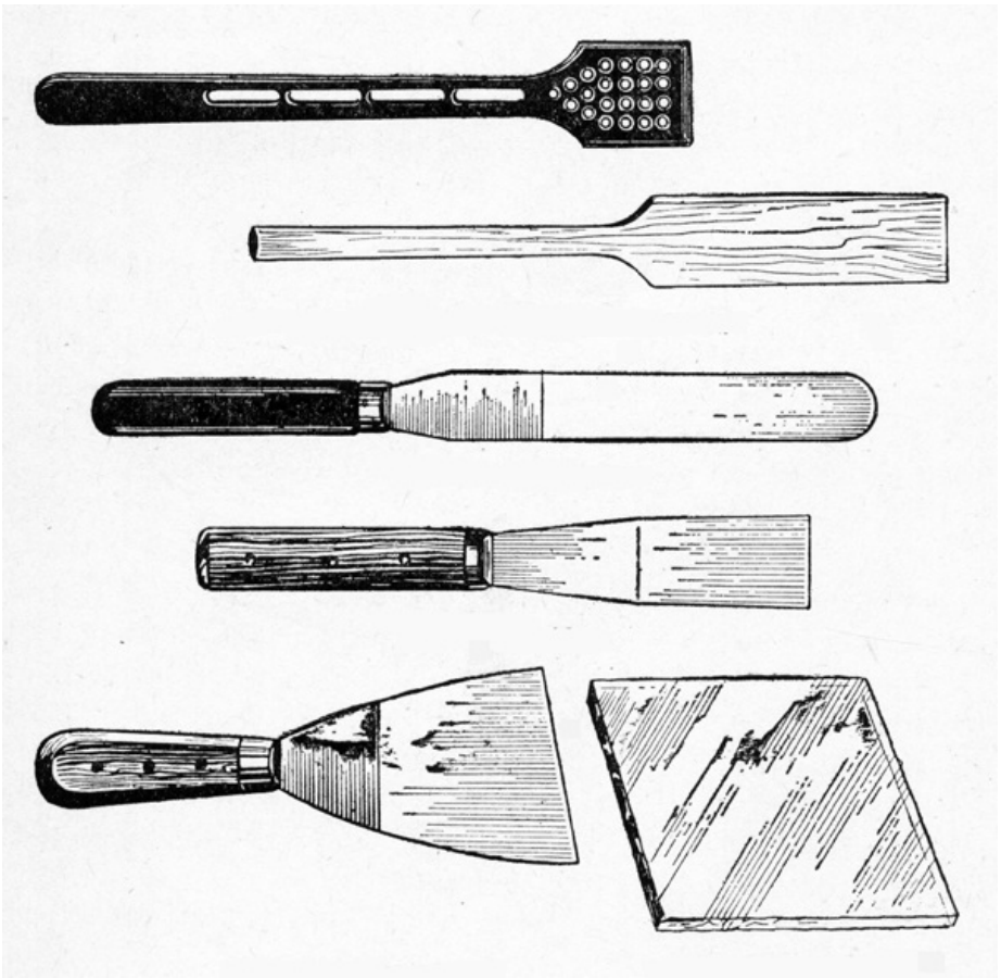
Iron and Wood Mixing Paddles Palette Knife Putty Knife Broad Scraper Glass Mixing Slab Plate 4.—Mixing Tools
