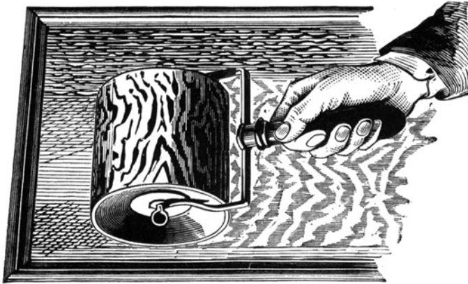
Fig. 28.—Oak Graining Roller in Use.
